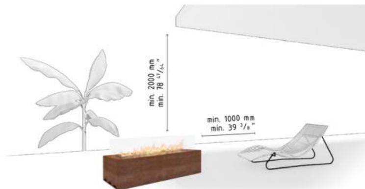
Picture 1: Minimum distance to flammable materials
