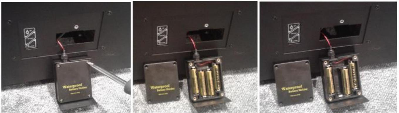
Photo 8: Replacing the batteries in the container
