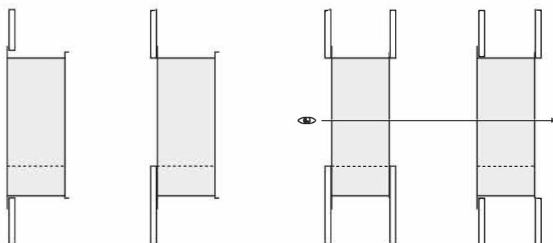
The XL and XXL are also equipped with metal pipes on top. These can be used to connect a tube to a ventilation outlet in order to lead the heat to the room. If these are not necessary or desirable in your application, they can easily be removed.
