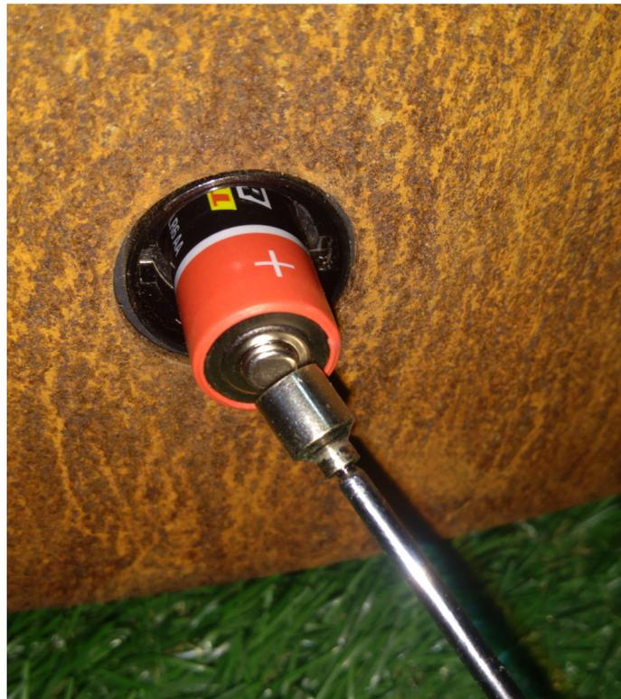
*Photo 6: Removing the first battery using the magnetic gripper*
