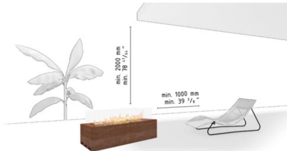
Figure 1: Minimum distance to flammable materials
